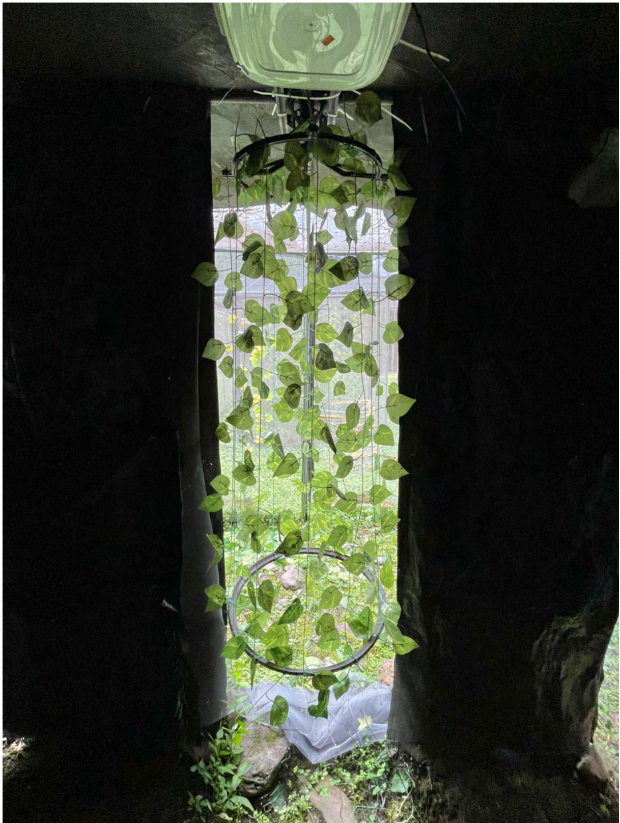
Figure S1 | Rotary obstacle apparatus as seen from the dark chamber of the experimental insectary. Top: modified optomotor machine. Left and right: opaque divider within the insectary, forming a bright slit.
